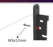
In order to connect the parts together properly, first insert the screw (1). then put nut inside the referenced nesting (2) then its safeto tighten screw (3).
