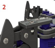
In order to make this connection easily we recommend placing the **M3 Nuts** first then use the **M3 x 12mm** to tighten it.
