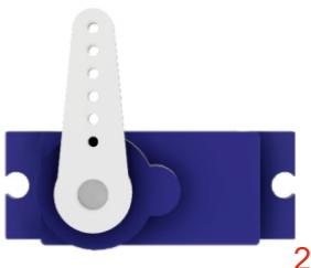
Remove the servo arm from the servo motor and reposition it perpendicular to the servo motor as shown.
