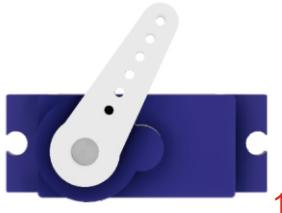
Attach the servo horn to the servo motor, then slowly turn the servo horn clockwise until it stops. It is not a problem if the servo horn is not the same as the angle shown in the image above. The important thing here is that you have hit the last note of the servo.
